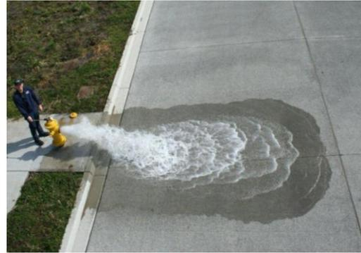
Pervious concrete permits a large volume of water to infiltrate through the pavement
