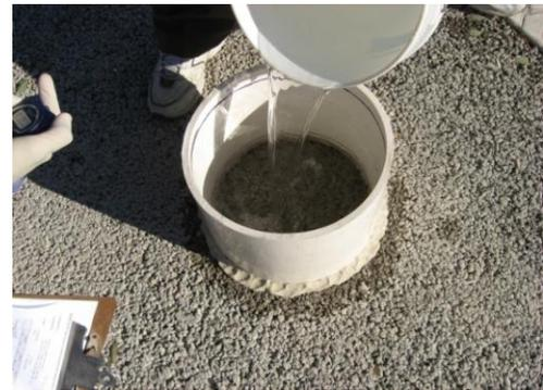
ASTM C1701 to evaluate the in-place infiltration rate of pervious pavement
